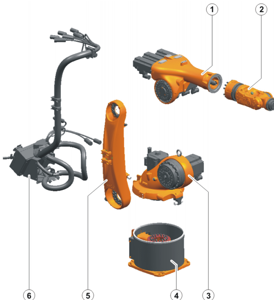
Fig. 3-2: Main assemblies of the robot
