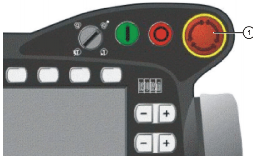
Fig. 3-3: EMERGENCY STOP button on the KCP
