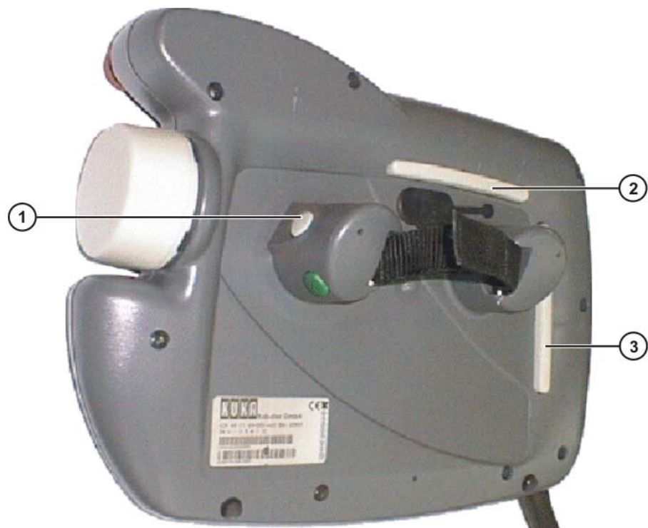
Fig. 3-4: Enabling switches on the KCP
