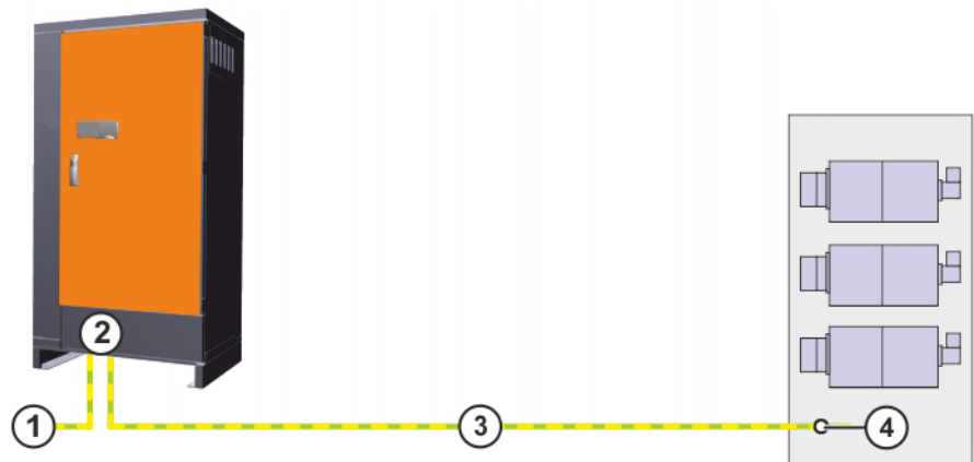
Fig. 6-20: Equipotential bonding, robot controller - robot kinematic system
