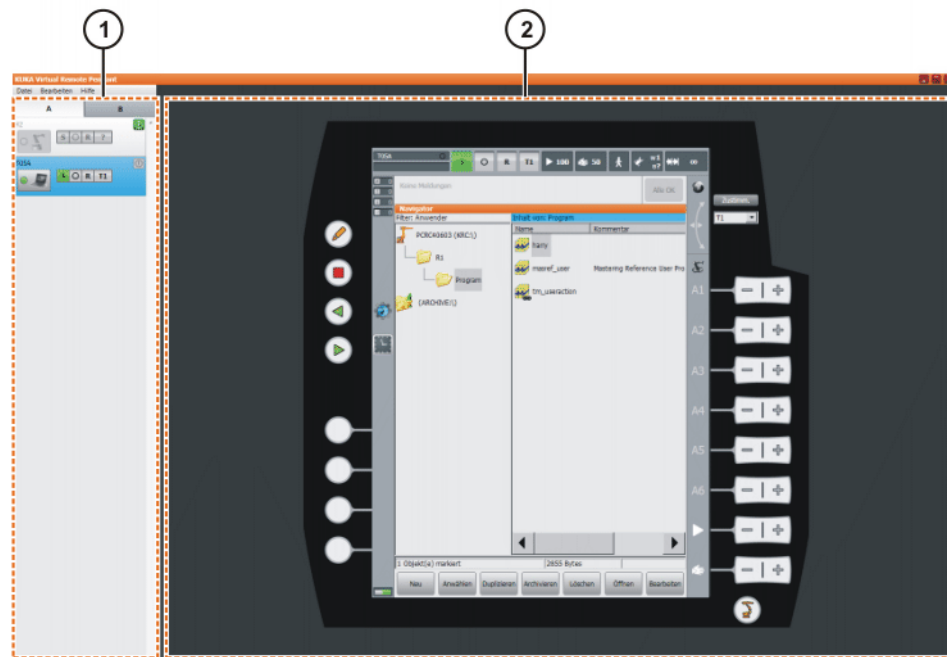
Fig. 6-1: KUKA.VirtualRemotePendant user interface
