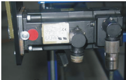
Fig. 5-3: Connecting the resolver cable to the resolver
