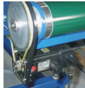
Fig. 5-3: Connecting the resolver cable to the resolver
