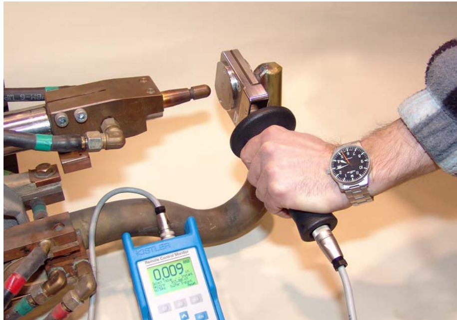
Fig. 6-4: Measuring with the force gauge
